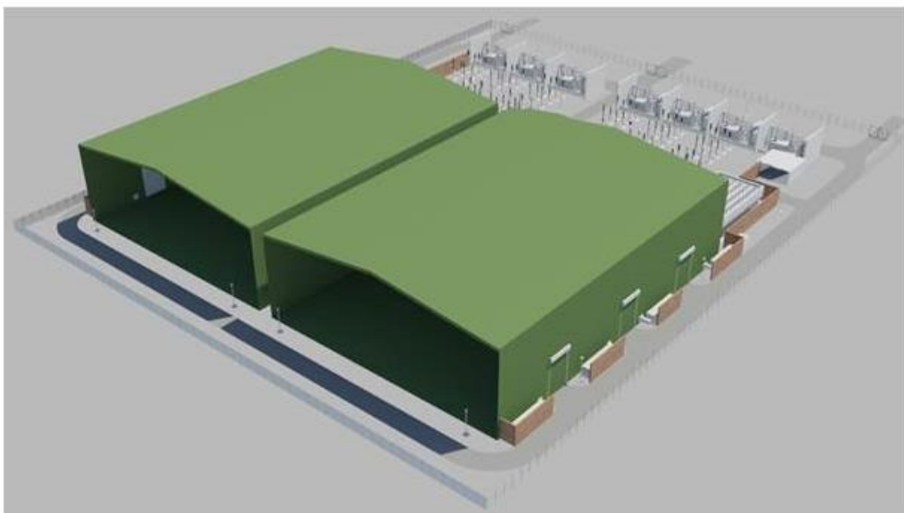
Diagram 5.22 Typical Layout of a 1000MW HVDC Converter Station
