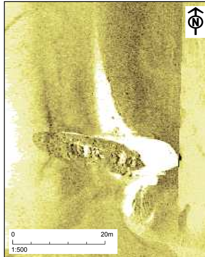
Sidescan sonar image of wreck 23.3m x 8.5m x 4.5m
