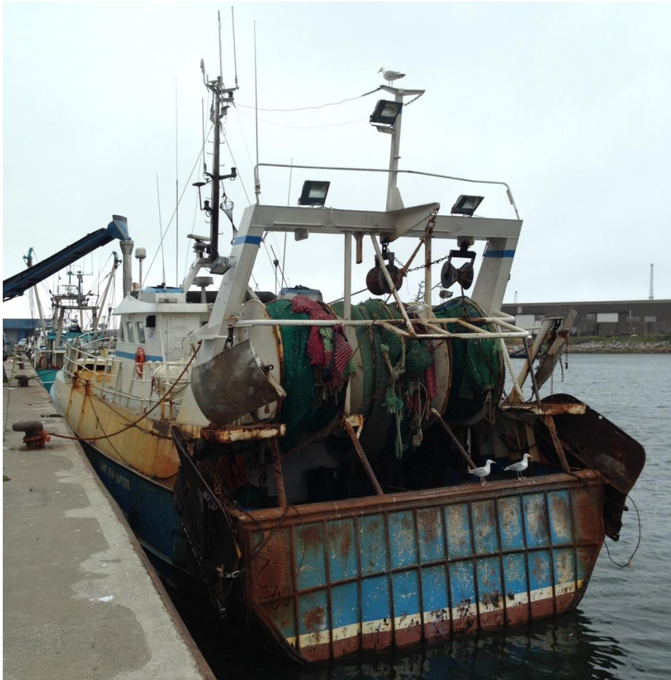
Plate 14.13 Example of a French Trawler carrying both Demersal and Pelagic Trawl doors.
