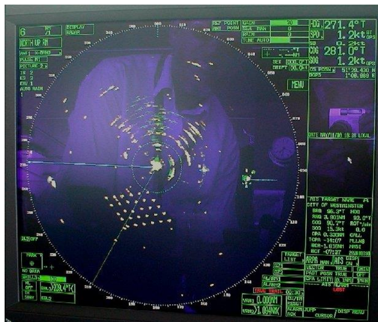
Figure 7.2 Illustration of typical ghosting produced on a passing vessel one n.m. from the wind farm boundary
