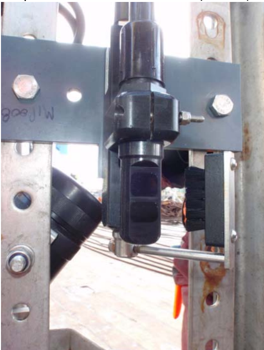
Seapoint OBS with Zebra-Tech Hydro-Wiper fitted to Cefas MiniLander
