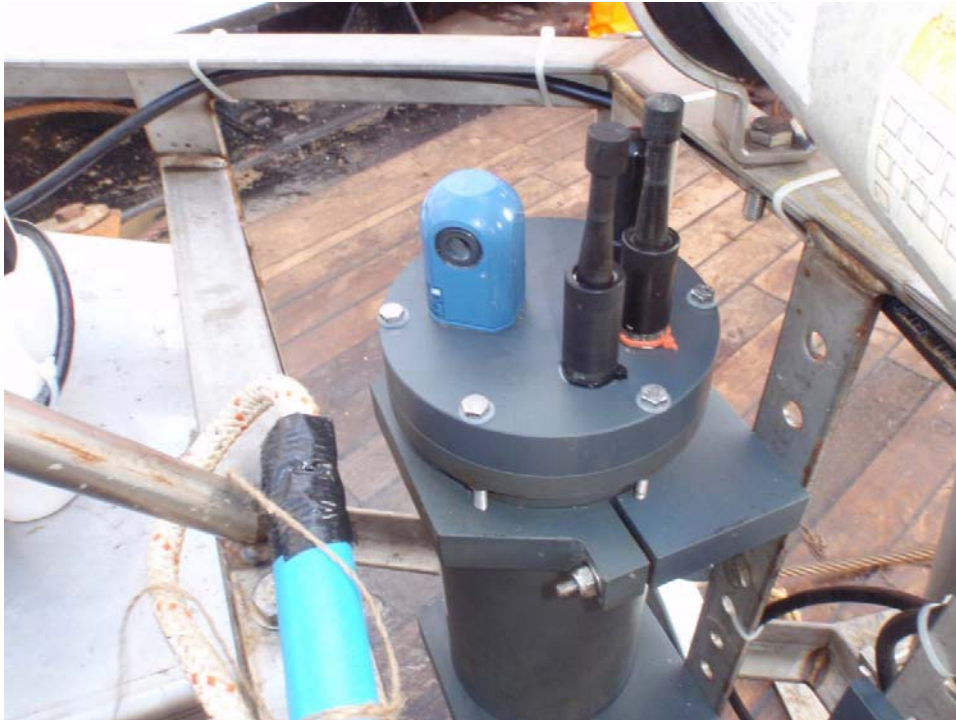
Cefas ESM2 logger with Aanderaa conductivity/temperature sensor fitted to Cefas MiniLander
