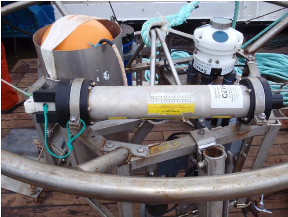
Acoustic release set-up on Cefas MiniLander
