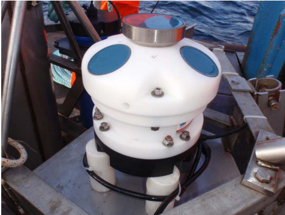
Nortek 600kHz AWAC AST fitted to Cefas MiniLander
