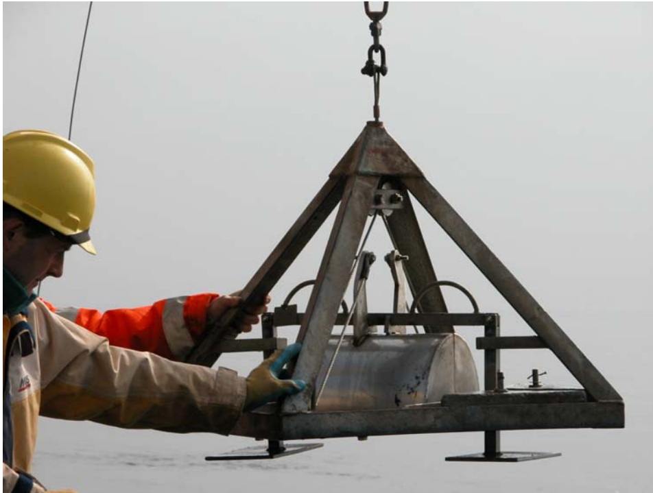
Cefas MiniLander fitted with Nortek AWAC, Booner tube, Seapoint OBS sensor, Cefas ESM2 logger and Applied Acoustics acoustic release
