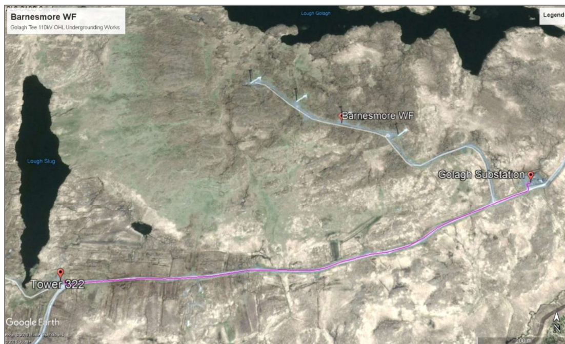
Figure 2 - Golagh Tee 110kV OHL Undergrounding Works
